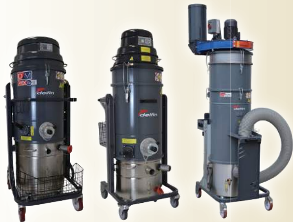
Delfin (Safety Management) Explosion-proof dust collection system for metal AM
