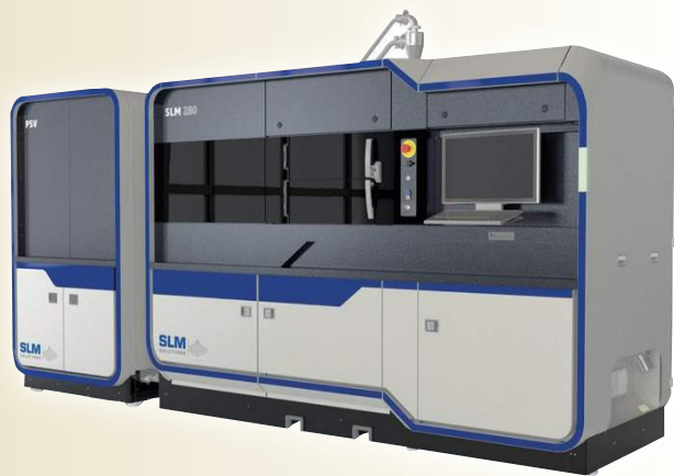
Nikon SLM Solutions (LPBF) Laser Powder Bed Fusion for high-precision, high-performance parts
