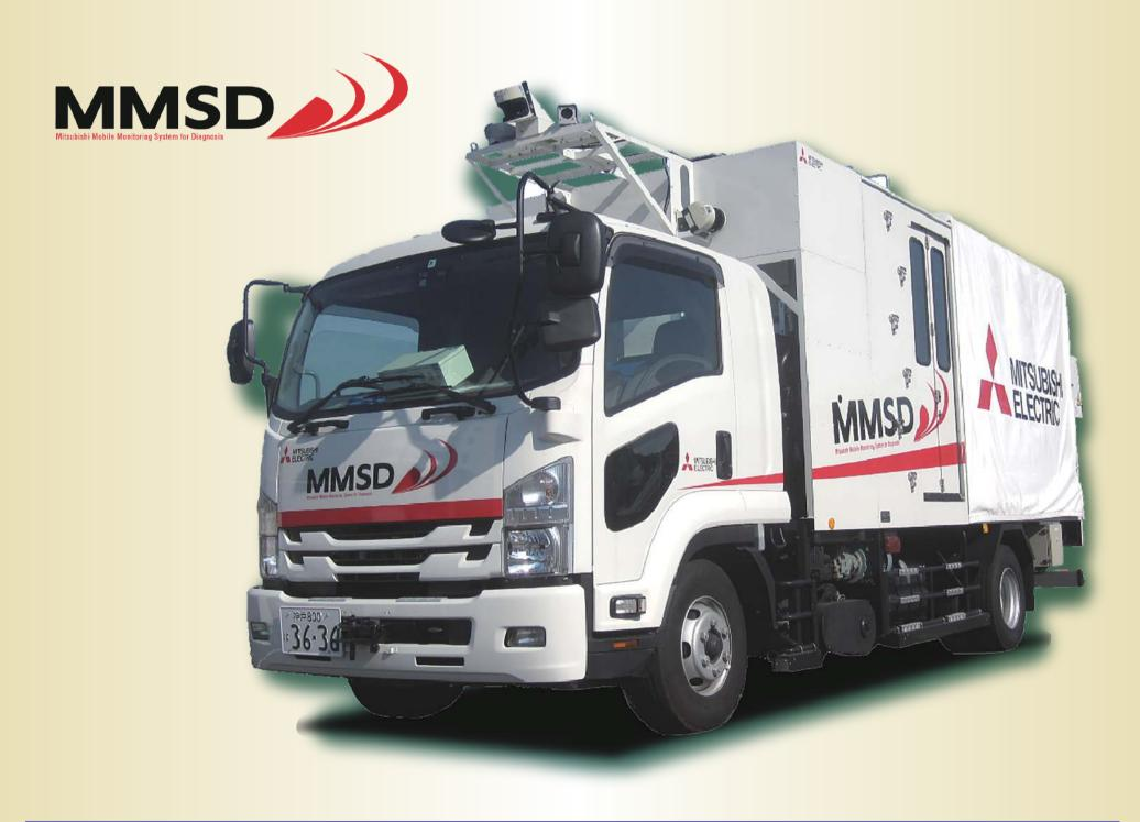
High density laser scanner, high resolution camera and various sensor technologies realize advanced automatic and labor-saving social Infrastructure inspections.
